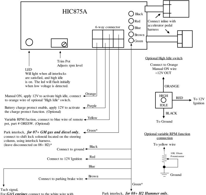
For *GAS engines* connect to the white wire with black stripe coming out of the bottom ECM X2 connector. For *Duramax diesel engines* connect to the white wire with black stripe coming out of the top ECM X1 connector.
